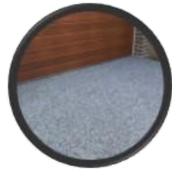
Figure 6 – Example of permeable concrete/ asphalt
